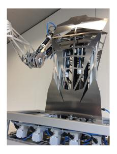
Biorobotic model of the human arm with two joints actuated by five monoand biarticular pneumatic muscles of different lengths and thicknesses. The robot considers non-linear lever arms and actuators with a nonlinear forcelength and force-velocity relation.
