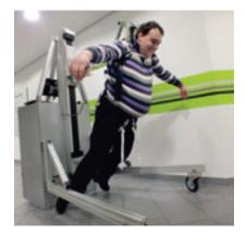
The displayed system allows the application of external mechanical perturbations to the body in order to study the motor control during complex walking.
